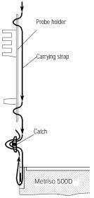
Fasten the carrying strap (14) and the two probe holders (12) and (13) as shown in the following figure. Make sure to fix the holder for the slim probe (10) at the left and the holder for the probe with lamp and pushbutton (9) at the right.
